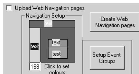
The colours of the background and the text are set by clicking either the background or the text shown on the diagram. Once clicked a colour selection window appears where the colours can be selected. The width of the events column can be adjusted by changing the default 168 to a large or smaller value.
